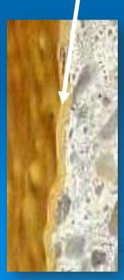
Spray applied epoxy w/ flexible polyurethane coating
