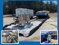
Secondary filters 50 & 5 Micron Water Sampled & Tested
