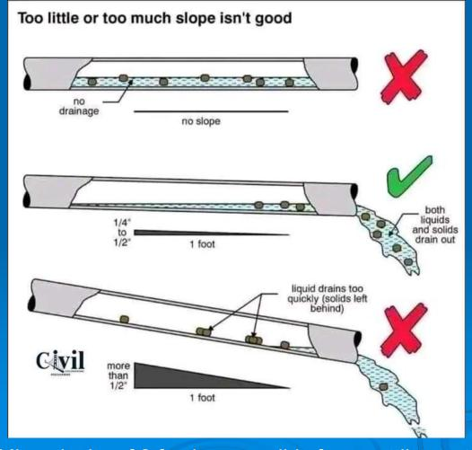
Min velocity of 2 fps keeps solids from settling out.
