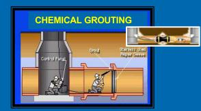
Chemical grout joint seal
