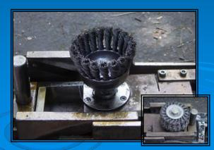
Router bit or wire cup brush – Brush smooth - Remove all coupons
