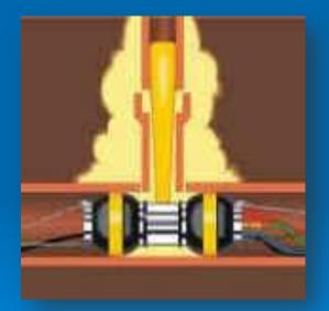
Chemical Grout to stop infiltration and stabilize the surrounding soil on the outside of the pipe
