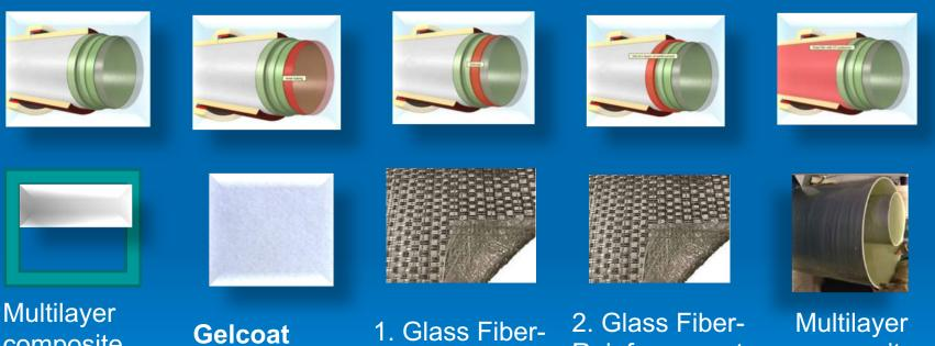
composite Clear plastic inflation tube w/Styrene Blocker (Removed after Curing) Gelcoat Resin impregnated Fleece
