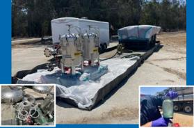
Secondary filters 50 & 5 Micron Water Sampled & Tested
