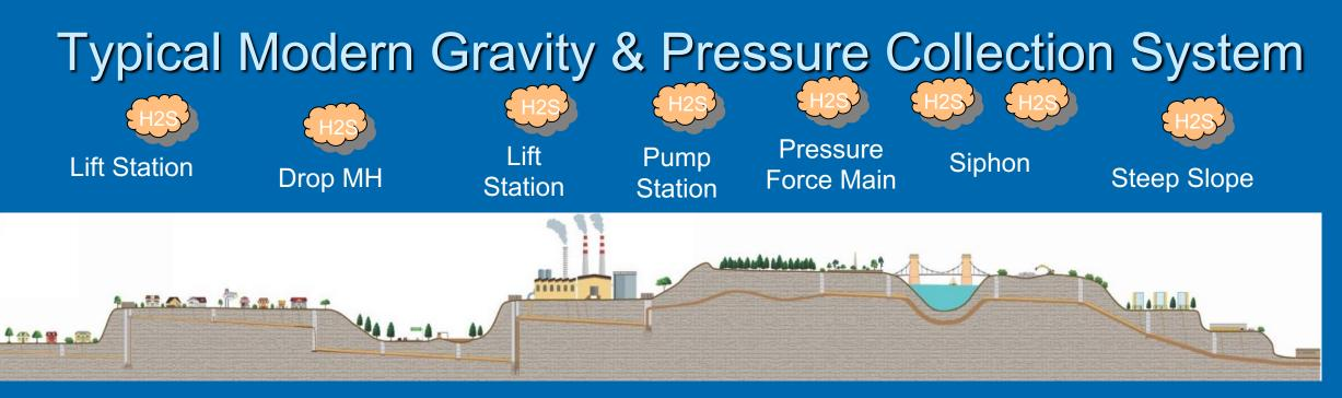
Min velocity of 2 fps keeps solids from settling out.
