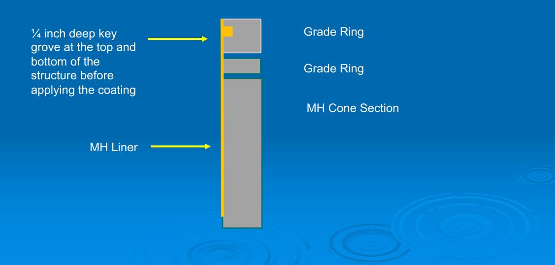
Trowel or Spray Apply Ridged or Semi Ridged Epoxy Protective Lining
