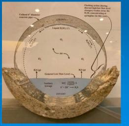
Corroded Concrete Pipe
